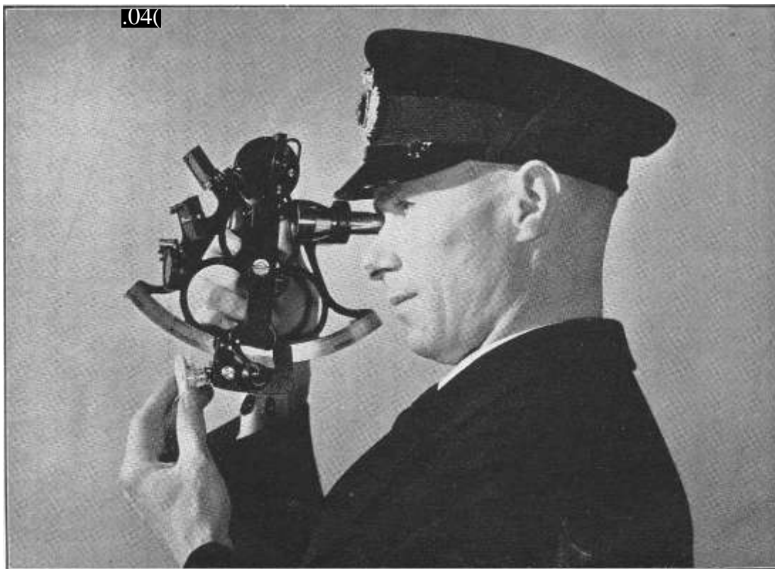
Fig. 11. The Sextant held in the normal position for taking sights.
