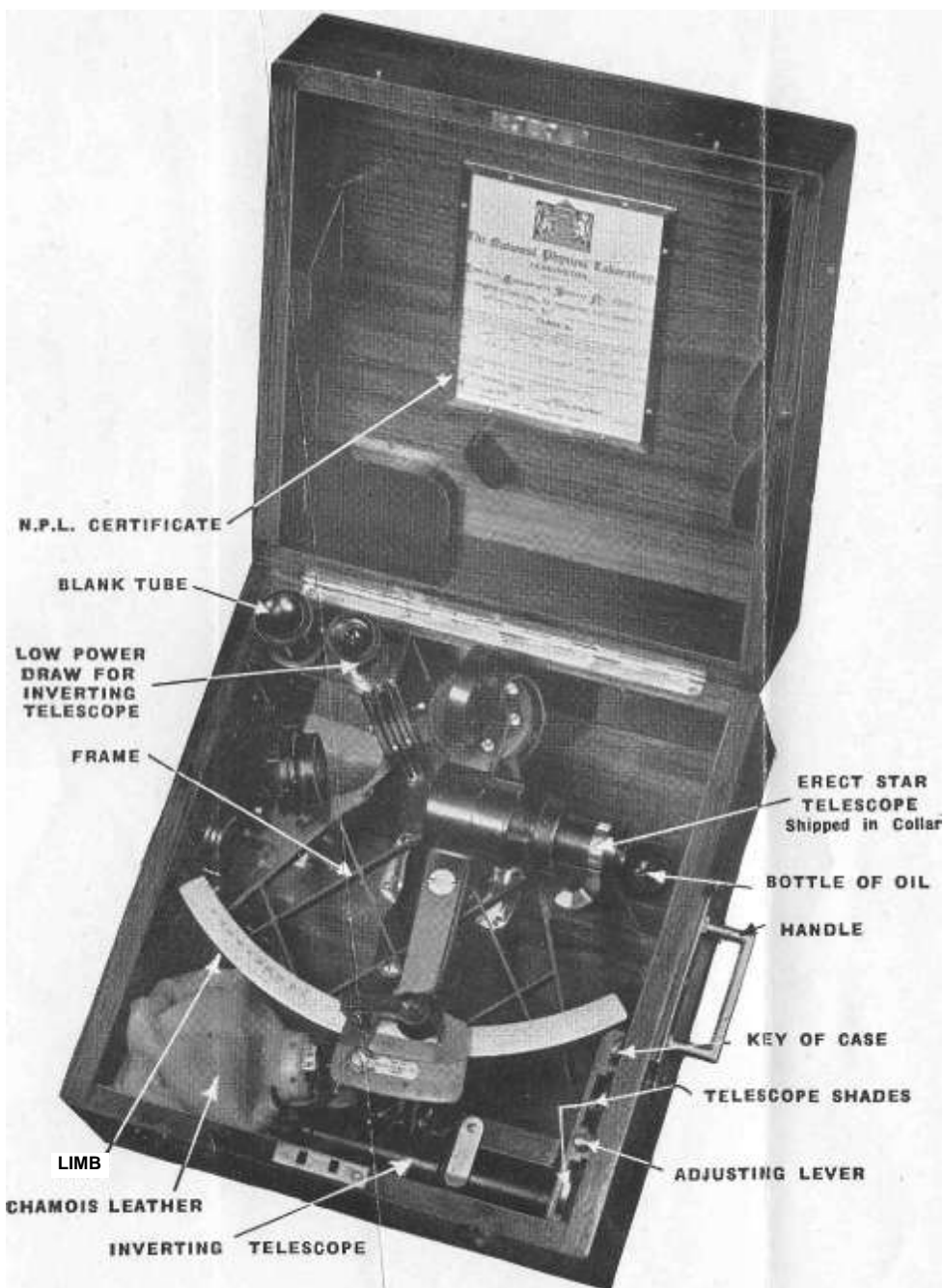
Fig. I. A Diamond Frame " Micrometer Sextant stowed in its case.
